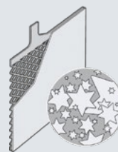
Without Carbon Boost® The plates are covered with sulfate
