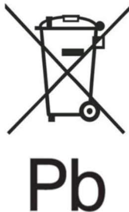
Figure 2 – Example of marking with symbol for separate collection according to Annex VI Part B and with the chemical symbol "Pb" for the heavy metal Pb content according to Articles 13.4 & 13.5
