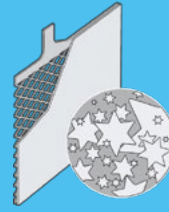
Without Carbon Boost® The plates are covered with sulphate
